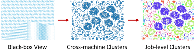
Fig. 3: LLM training job recognition procedure of LLMPPrism in training clusters with 2,880 GPUs in Platform-X.
